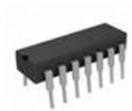
Texas Instruments SN7402N Quad NOR or equivalent.
