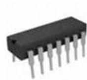
Texas Instruments SN7404N Hex Inverter or equivalent.
