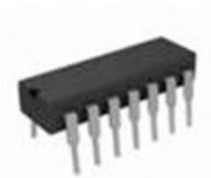
Texas Instruments SN7400N Quad NAND or equivalent.
